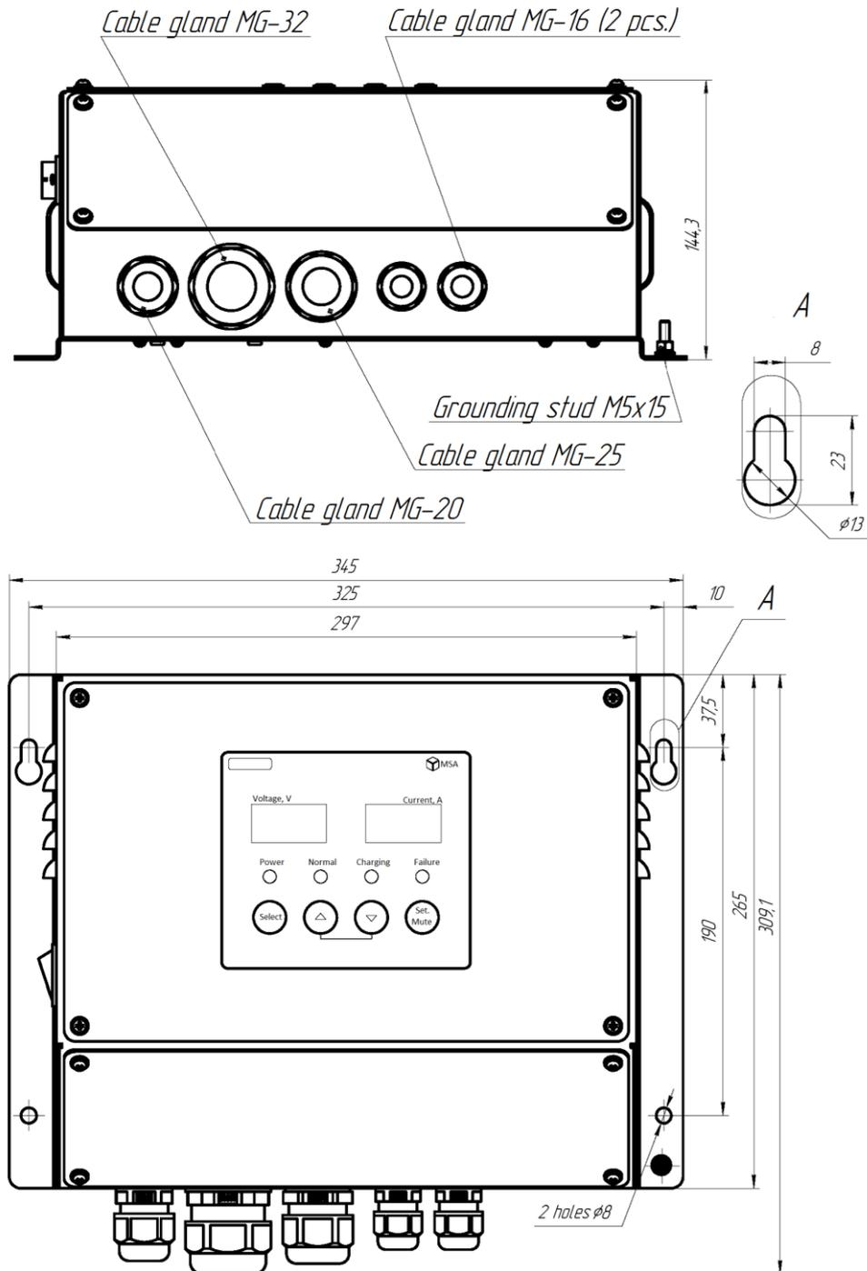
Figure A.1 – CH-105, CH-105-24 outline and installation dimensions
