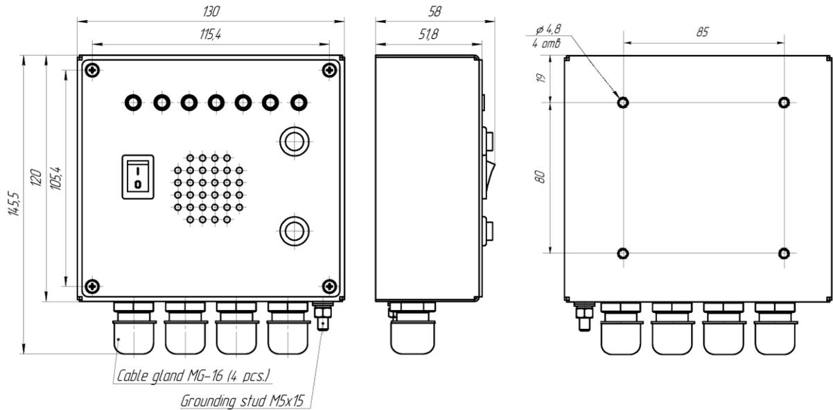
Figure B.2 AU-206 outline and installation dimensions
