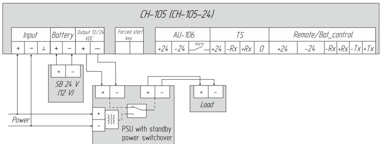
Figure 6 – Load connection using separate PSU
