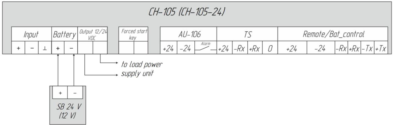
Figure 5 – Diagram of load to SB switched connection
