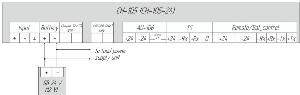
Figure 4 – Diagram of load to SB direct connection
