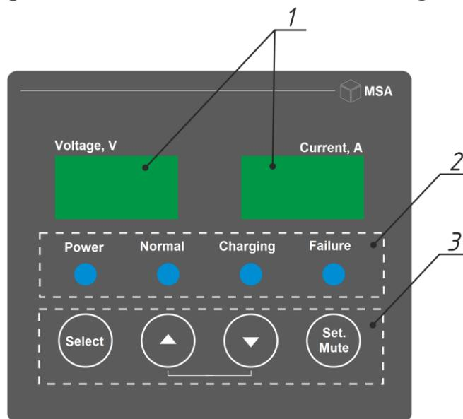
Figure 2 – Control and display panel
