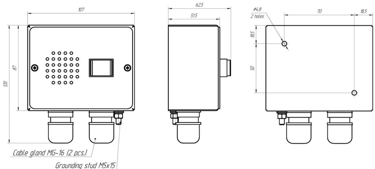
Figure B.1 – AU-106 outline and installation dimensions
