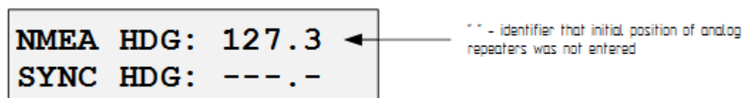
Figure 10 – the Product's display when initial position data of analog repeaters are absent
