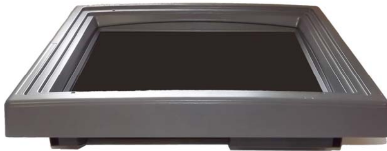
Figure 11. Appearance of LCD display prepared for installation and inserted into the frame
