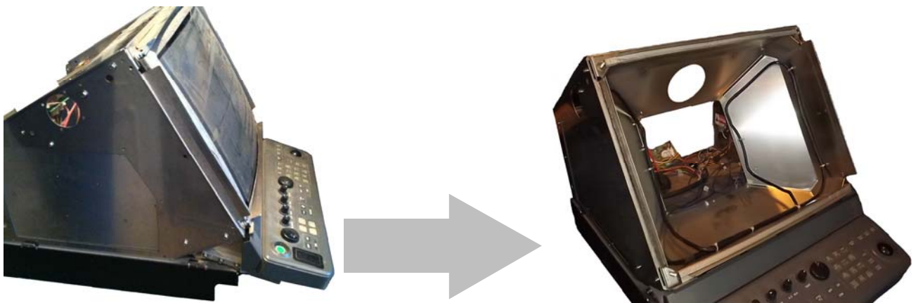
Figure 5. Dismantling CRT from radar rack
