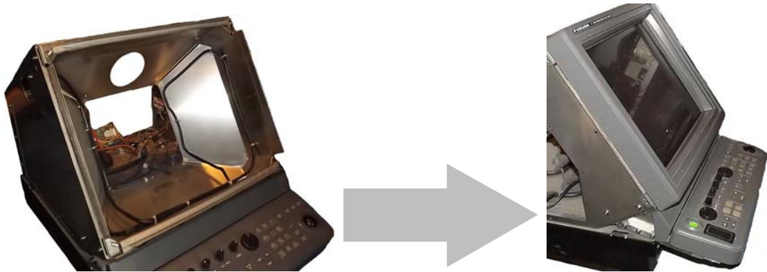
Figure 12. Mounting display into radar rack
