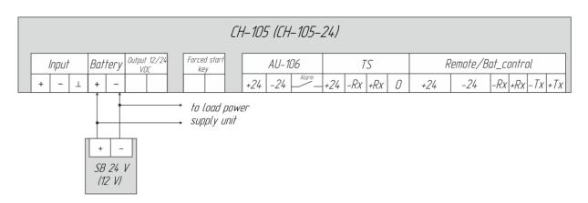
Figure 4 – Diagram of load to SB direct connection
