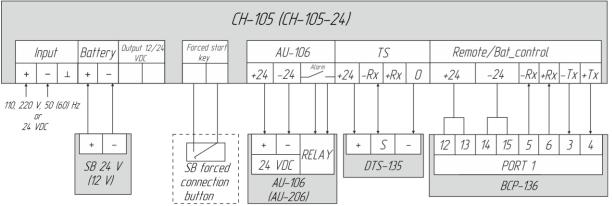
Figure 3 – The Product's connection diagram
