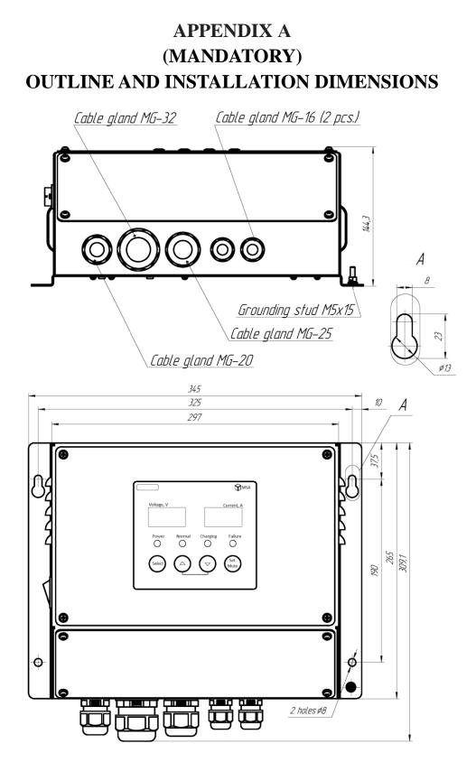
Figure A.1 – CH-105, CH-105-24 outline and installation dimensions
