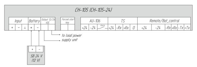
Figure 5 – Diagram of load to SB switched connection
