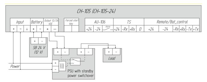
Figure 6 – Load connection using separate PSU
