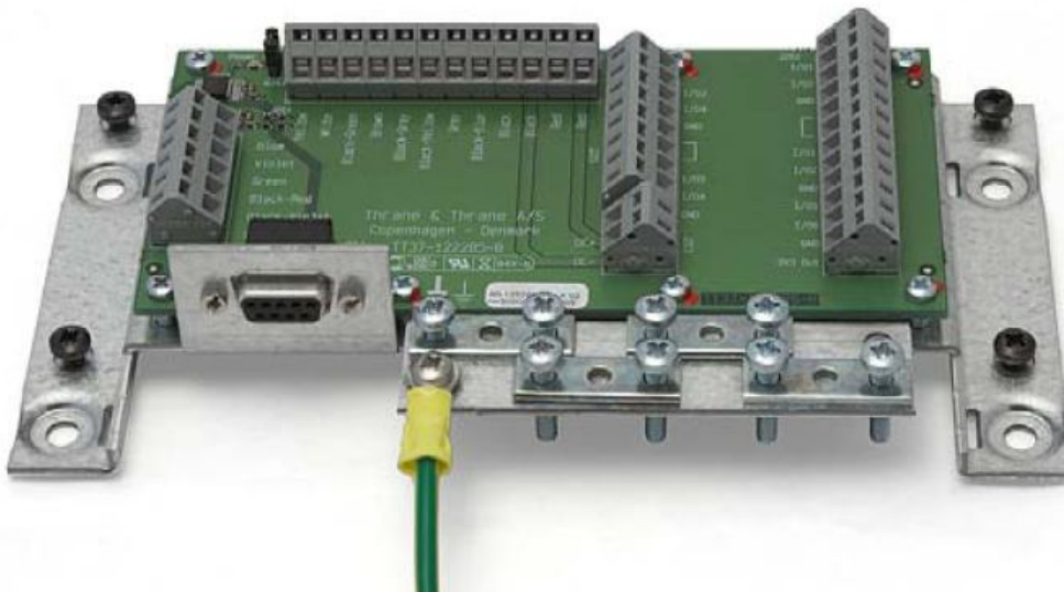
Fig. 5. Connecting the earthing lead to the SCB-133
