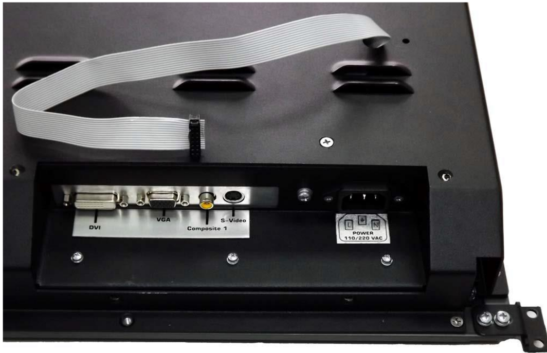
Figure 15 – Location of connectors and control cable in LCD display
