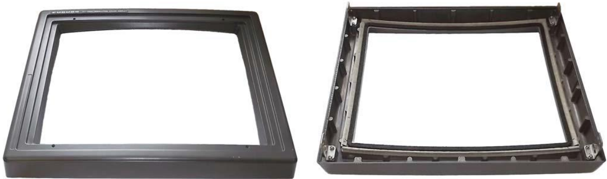
Figure 4 – CRT frame view (removed from radar rack)
