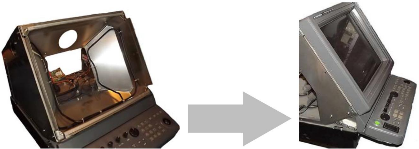
Figure 12 – Mounting display into radar rack
