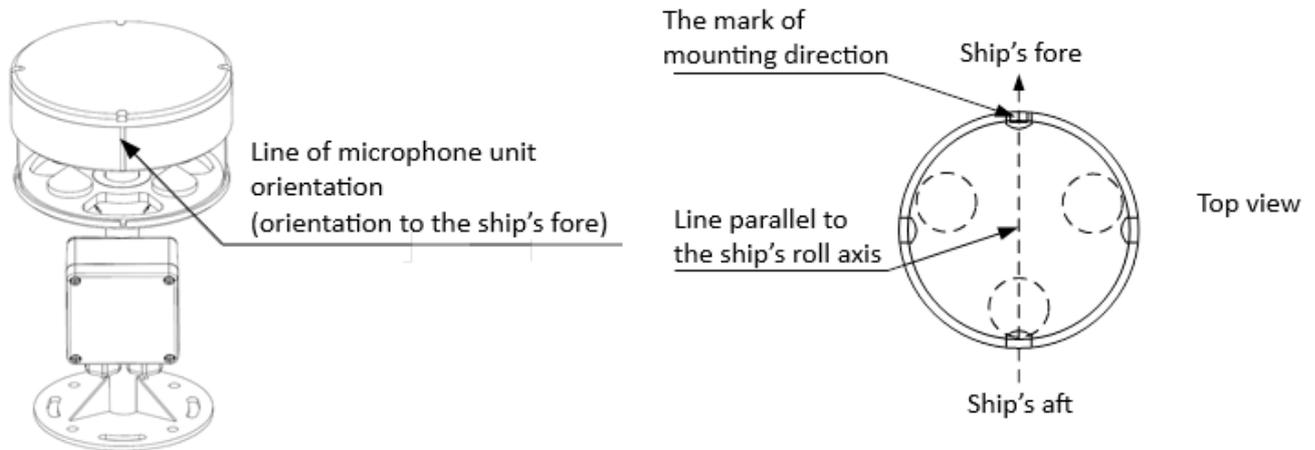
Figure B.1 – MU orientation at mounting
