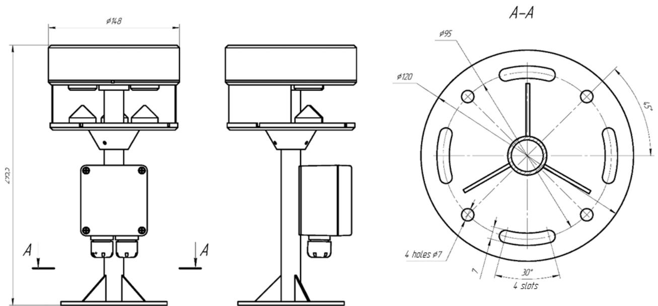
Figure A.3 – Outline and installation dimensions of NS-201M
