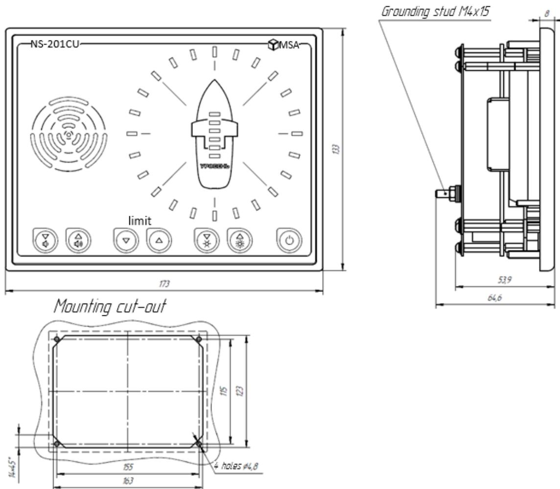
Figure A.1 – Outline and installation dimensions of NS-201CU (NS-201R)
