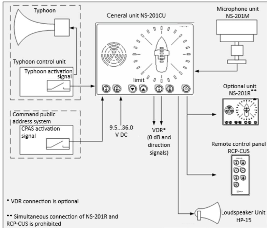
Figure 4 – The general connection diagram of the SC and external devices
