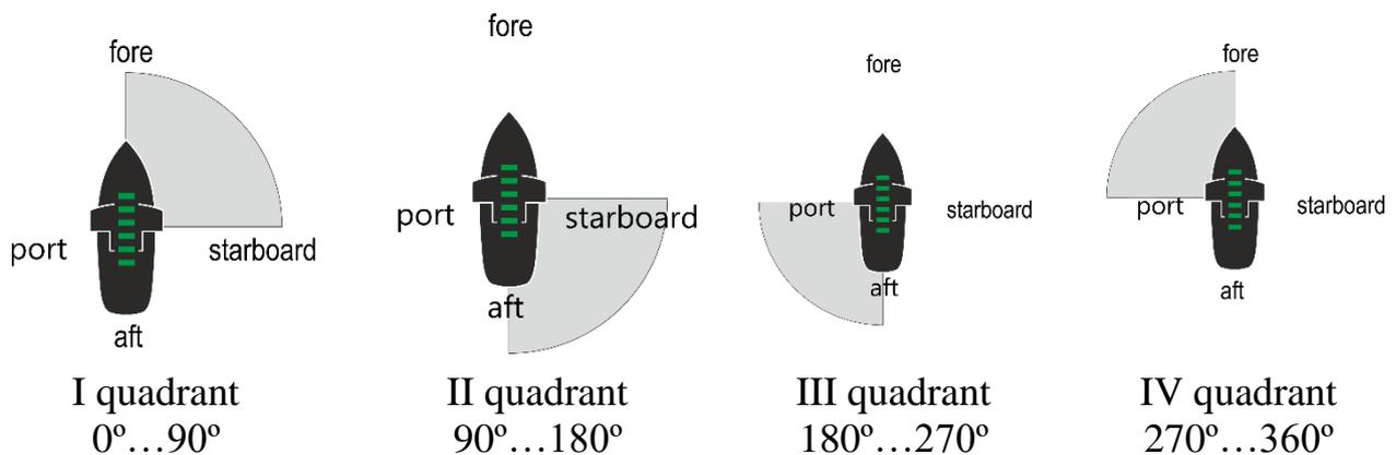
Figure 1 – Direction of signal source (fixed sector)
