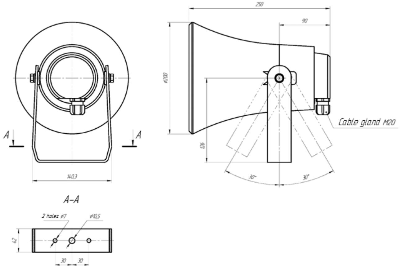
Figure A.2 – Outline and installation dimensions of HP-15
