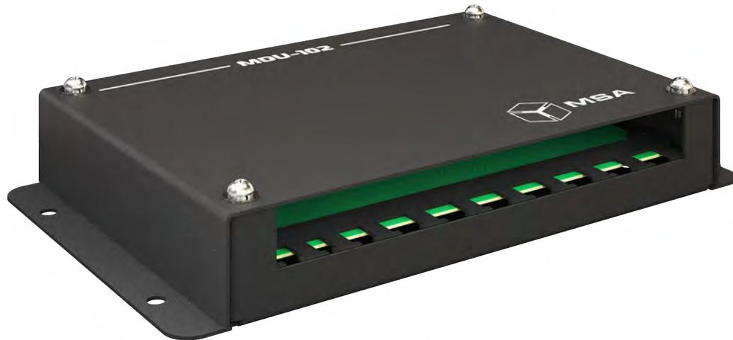
The MDU-102 is designed for the multiplication of NMEA 0183 signals, version 1-3 (IEC 61162-1, 61162-2) or other serial data transmissions via RS-232 and RS-422/485 interfaces from one or two sources. The unit provides a checksum test for data received on the first channel.
