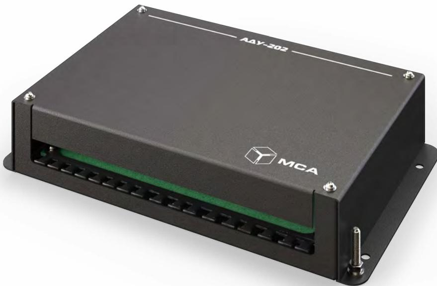
The ADU-202 is designed for the amplification and multiplication of NMEA 0183 signals, version 1 and 2, or other serial data transmissions via RS-232 and RS-422/485 interfaces. An integrated summarizer combines the input NMEA 0183 sentences and transmits the results to one or two output groups, depending on the jumpers' position on the printed circuit board.
