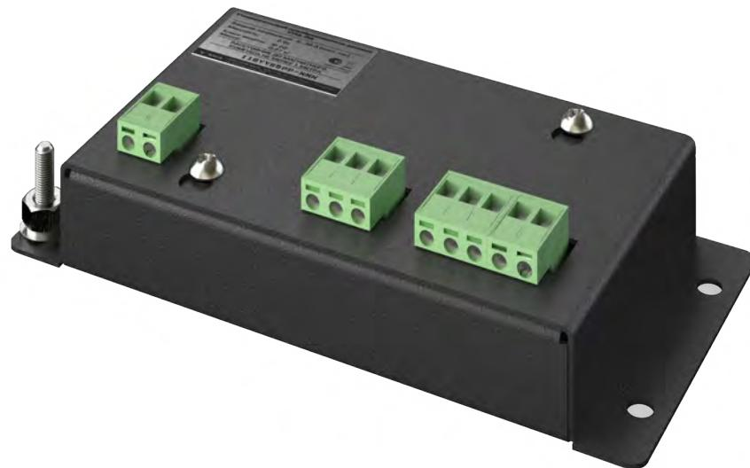
The DFR-118 data converter processes received NMEA data and repeats them to units connected to the converter output port. Depending on the software used, the unit is capable to filter and change baud and frequency rate of the data stream, adjust letter and digit of the NMEA sentences and add a checksum.
