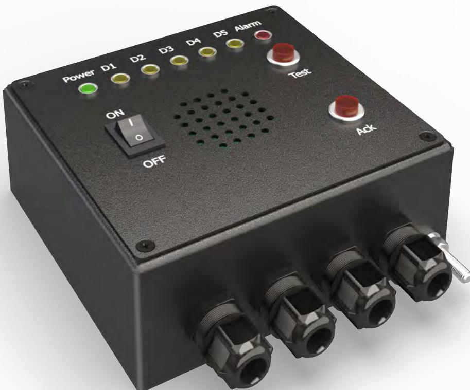
The AU-206 alarm unit controls the activation of external alarms on up to five simultaneously connected devices, having a dry contact type output. Triggered at least on a single output, an alarm causes sound/visual signal and closing of "power" output contacts, where external alarm devices may be connected (e.g. lamps, loudspeakers, etc.).
