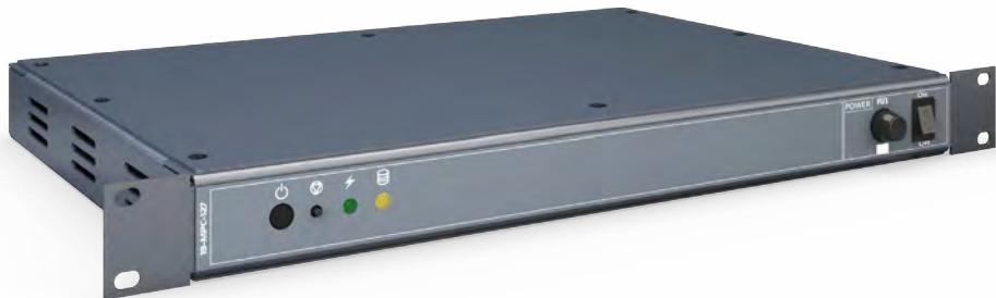
The 19-MPC-127(1U) marine computer unit can be used for process control, electronic mapping, automation systems, etc. The unit is designed to fit into a 19" rack. The unit can operate both with 24 VDC or 110/220 VAC. The 19-MPC-127(1U) designs are offered with various numbers of network and COM-ports. The VGA interface is used to display graphic data. The device has a galvanic isolation from power mains.
