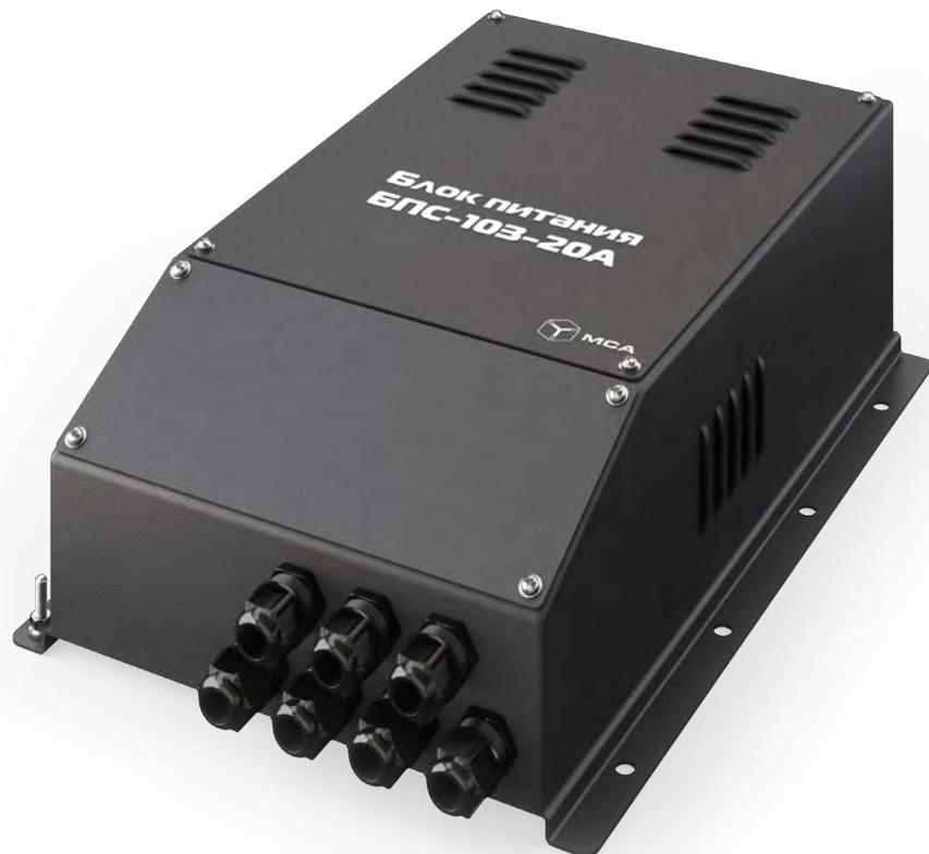
The PS-103-20 with a rated power of 192 W is designed to operate with 110 (optionally) / 220 VAC and provides unregulated power of 24V for various shipboard and industrial equipment. The PSU has an input for a standby storage battery (24 VDC) with an automatic switchover in the event of a main power supply failure. A power loss actuates the closing of built-in dry relay contacts.
