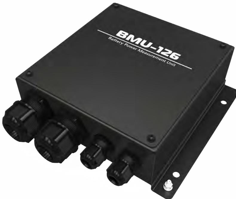
The BMU-126 reads the actual current and voltage data of a storage battery. Charge/discharge current and voltage may be controlled remotely using third-party devices. Readings are transmitted to the BCP-136 battery control panel via an RS-422 interface.
