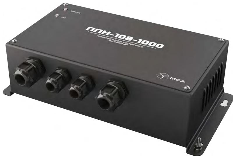
The DC-108-1000 operates with the mains of 24 VDC, converts the input voltage into a regulated VDC and protects electronic equipment against input voltage surges and peaks. The rated power is 960 W.
