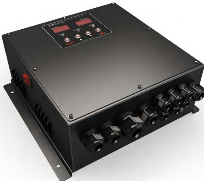
The PCH-205 power supply / automatic battery charger is designed to operate with single-phase mains 50-60 Hz 110/220VAC and provide 24VDC to shipborne systems and other industrial equipment with a total capacity of up to 1000 W. Combined with power supply, the PCH-205 charges connected storage batteries automatically. In case of a main power failure the unit switches the load to the storage battery automatically.
