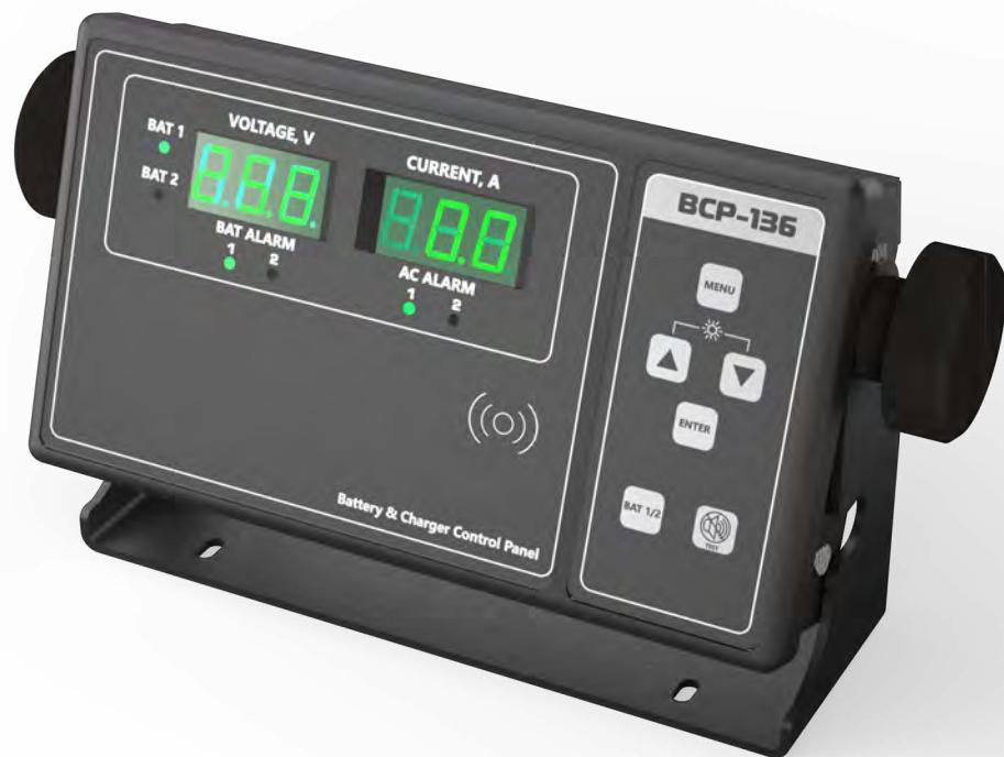
The BCP-136 allows remote setting of power supply units/battery chargers CH-105 and PCH-205. The device controls the status of connected storage batteries, indicating current charge/discharge and voltage data. In case of a power voltage failure and battery discharge the BCP-136 triggers sound and light alarm.
