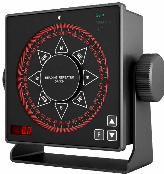
The DR-309 steering repeater displays the vessel's course data received in NMEA-sentences from various digital sources using a card and LED indicator. The device rebroadcasts the received NMEA data through an RS-422 (or CAN optionally) interface.
