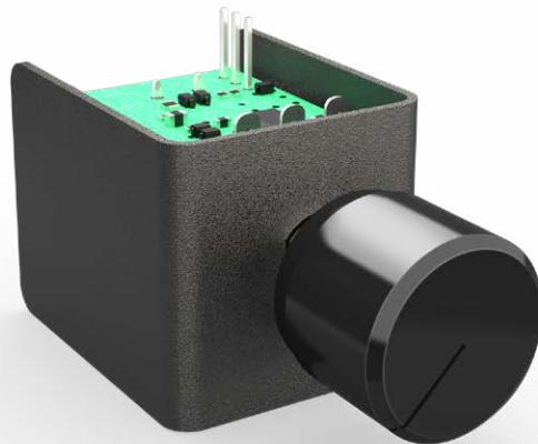
The DM-107 dimmer is a low-voltage power regulator for DC circuits, designed for a smooth adjustment of load power by potentiometer rotation. The load may be resistive (lighting lamps, resistors, etc.) and inductive (solenoids, valves, engines, etc.).
