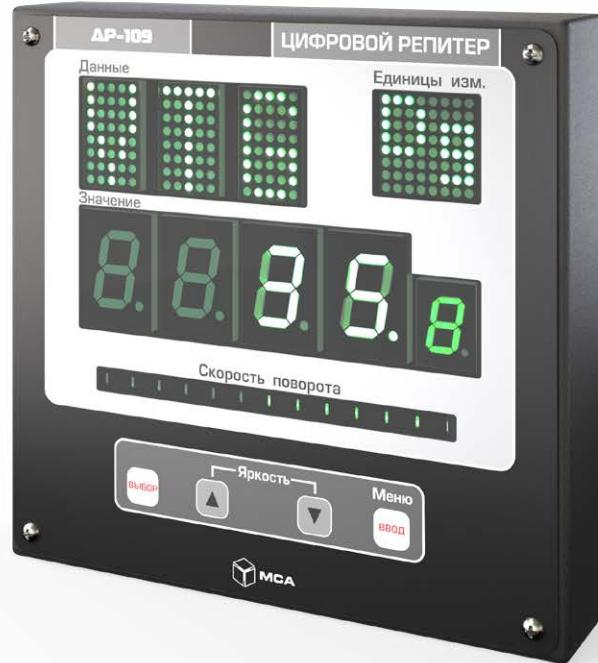
The DR-109 multipurpose digital repeater allows the visual indication of digital data received in NMEA 0183 sentences through RS-232 and RS-422/485 serial interfaces. The DR-109 provides sequential displaying of up to 3 data types on the built-in LED indicator (ship speed and heading, depth below keel, current time and weather conditions). The data of ship turn rate may be displayed regardless of main data on the built-in LED linear.
