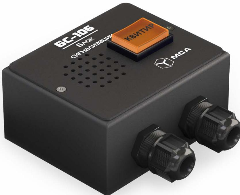
The AU-106 alarm unit provides a sound and visual signal, when triggered. The activation is ensured by closing (opening) dry contacts or voltage levels.
