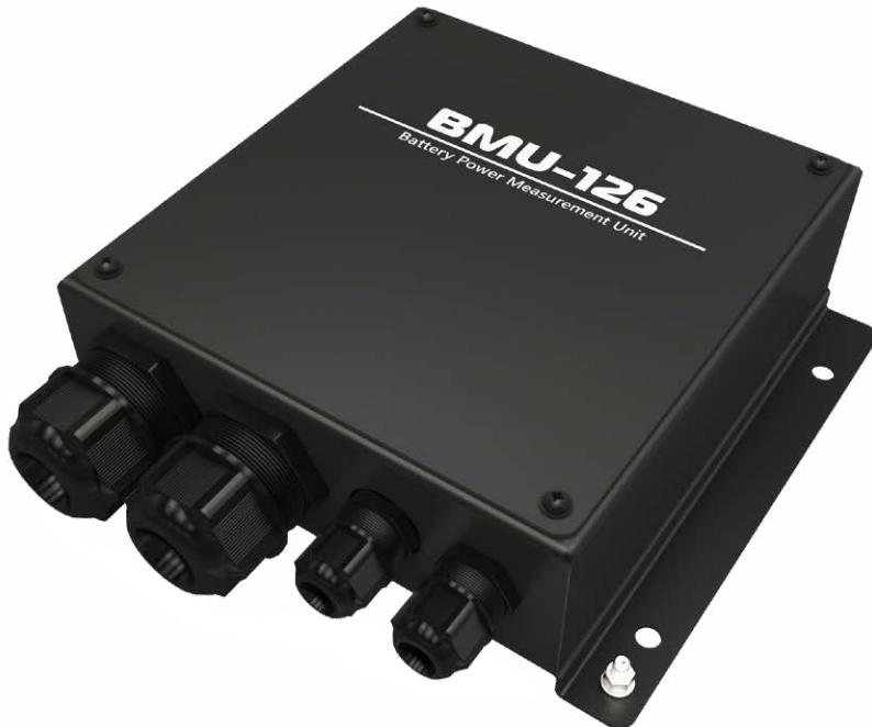
The BMU-126 reads the actual current and voltage data of a storage battery. Charge/discharge current and voltage may be controlled remotely using third-party devices. Readings are transmitted to the BCP-136 battery control panel via an RS-422 interface.
