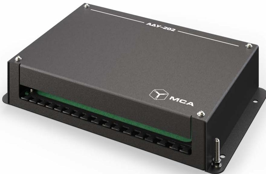
The ADU-202 is designed for the amplification and multiplication of NMEA 0183 signals, version 1 and 2, or other serial data transmissions via RS-232 and RS-422/485 interfaces. An integrated summarizer combines the input NMEA 0183 sentences and transmits the results to one or two output groups, depending on the jumpers' position on the printed circuit board.
