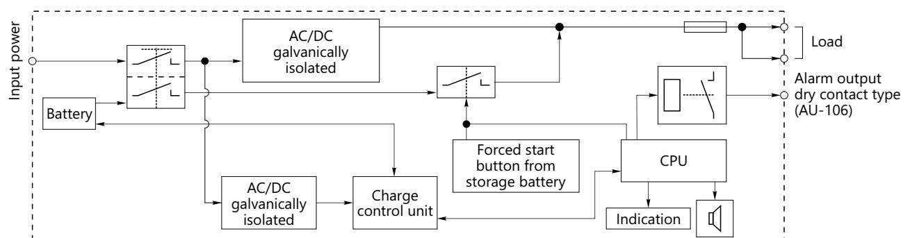
Power supply unit (built-in storage battery)
