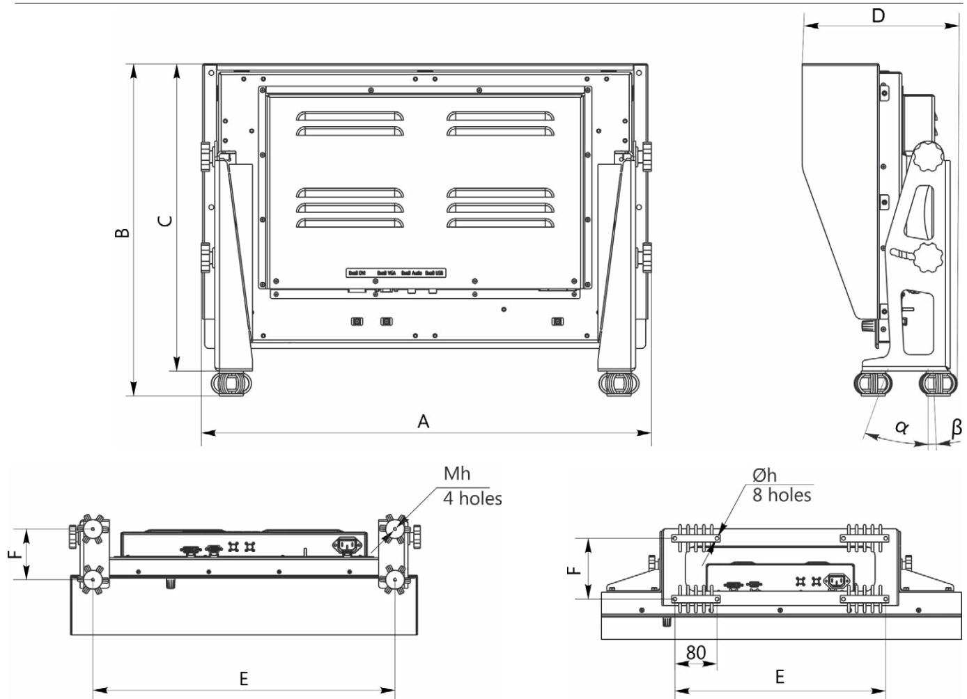
**Mounting holes location if mounted on a bracket with vibration isolators (Type 1)**
