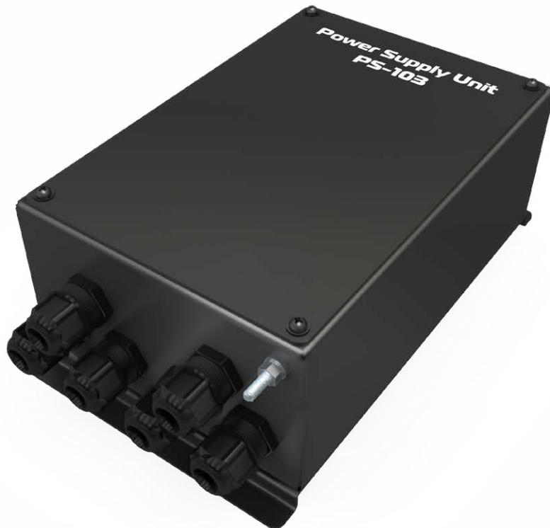
The PS-103 power supply unit with a rated power of 192 W operates with 110 (optional) / 220 VAC and provides unregulated power of 24V for various shipboard and industrial equipment. The PS-103 has an input for a standby storage battery (24 VDC) with automatic switching in the event of a main power supply failure. A power loss actuates the closing of built-in dry relay contacts.
