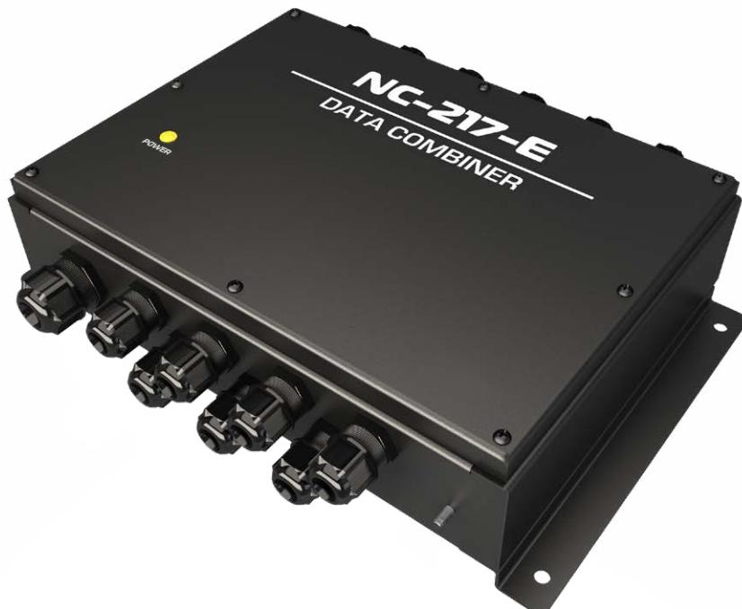
The NC-217 receives NMEA 0183 messages via four RS-232/422 inputs, combines them according to the customer settings and repeats them via twelve RS-232/422 outputs. Two additional bidirectional service ports and 1 USB are provided.
