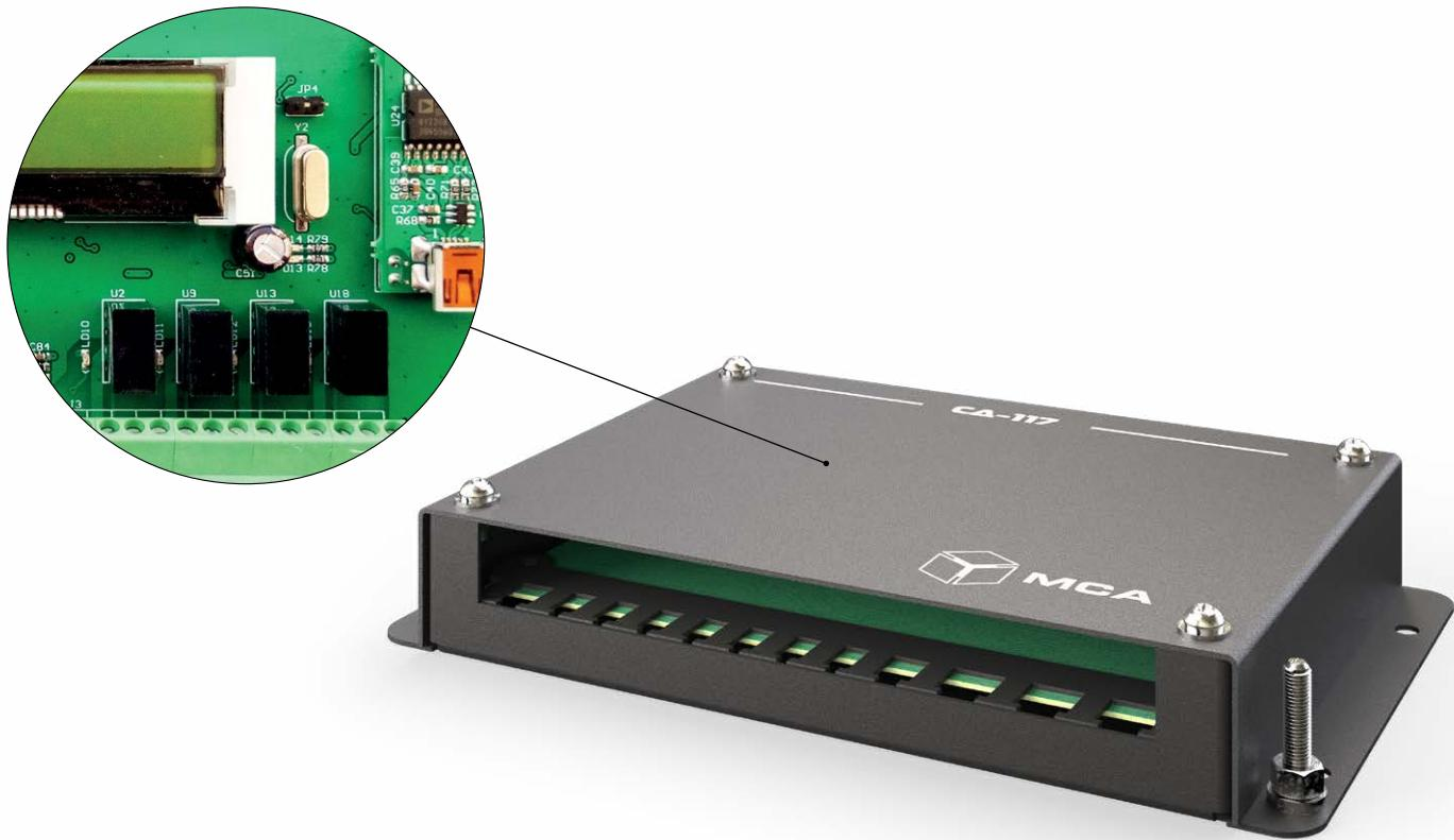
The NC-117 receives NMEA 0183 messages via eight RS-232/422 inputs and 1 USB port. It combines the received messages according to the customer settings and repeats them via four RS-232/422 outputs and 1 USB port.
