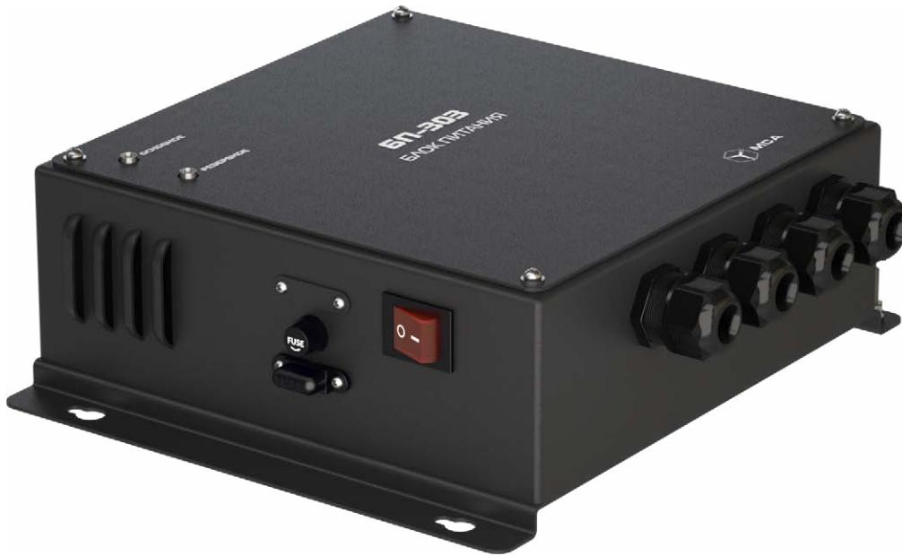
The PS-303 power supply unit operates with 220VAC or 24/12 VDC and converts the input voltage into a regulated voltage of 12/24 VDC. The unit has an input for a standby power source of 12/24 VDC, which switches over automatically in the event of a power supply failure.
