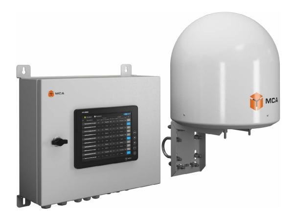
AHS-1022 is designed for low temperature protection and automatic heating of antennas exposed on open deck. Antenna heating unit (AHU) is an insulated radome with built-in (inside) heaters and temperature sensors.
