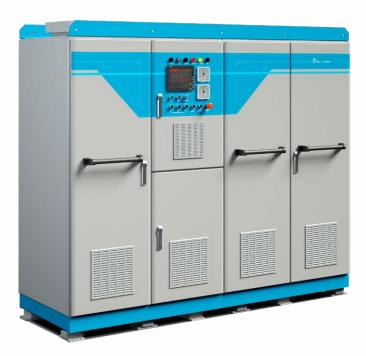
Voltage converter with pulse width modulation and active rectifier is based on high-power IGBT transistors. SEMIKRON power converter assemblies, which are highly resistant to harsh environmental conditions and temperature cycling, are used as transistors.
